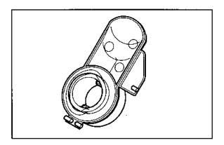
Maintaining pressure on the water circuit adapter, turn latch clockwise to lock and seal water circuit adapter onto MPS console.
